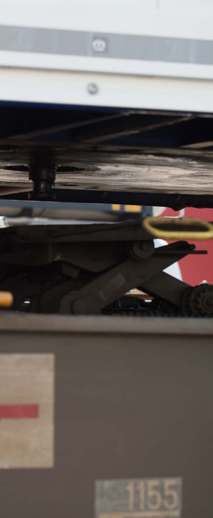
4:48 p.m.: Tutto bene. The trailer is securely fastened to the pocket wagon.
