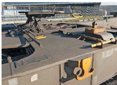
A triple height-adjustable king pin box to anchor semi-trailers to the newest-generation T3000e pocket wagons, in the highest (left) and lowest positions.
