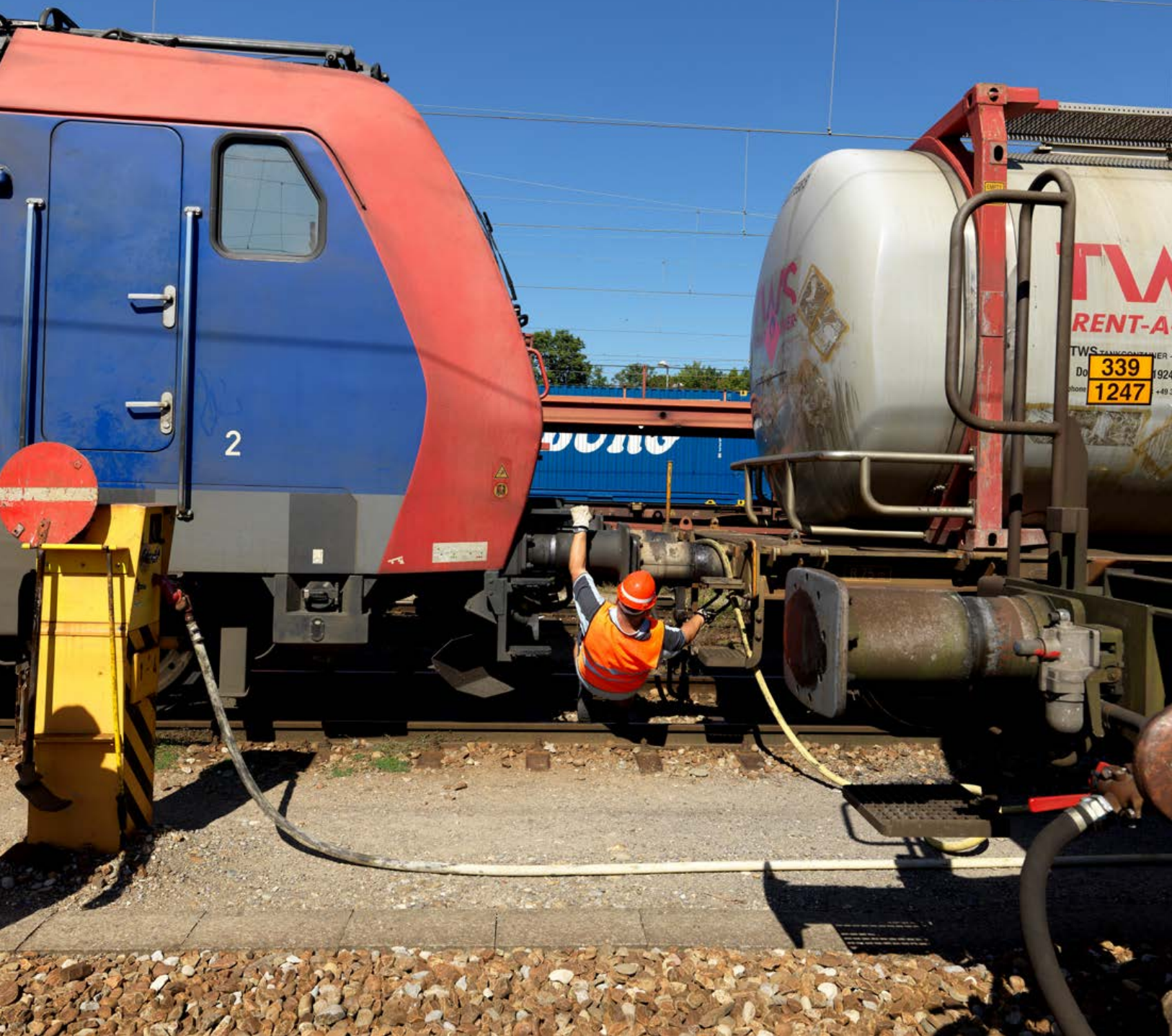
14:49 p.m.: A change of locomotive. Locomotive Type 482 is shorter and lighter than Type 47, but as a so-called multi-system locomotive, it is equipped with IT for both the Swiss and the German railway networks. The next engine driver, Uwe Anders, couples the locomotive to the train himself.
