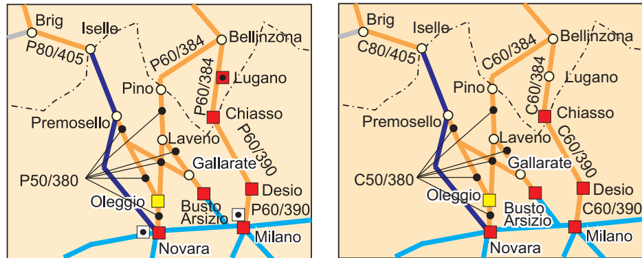
Example of codified routes from Switzerland to Northern Italy Left: for semi-trailers (P = poche) Right: for swap bodies (C = caisse mobile)
