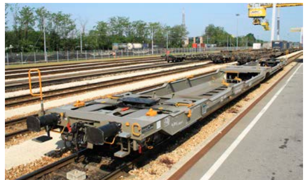
The T3000: a 6-axle double pocket wagon, 2014
