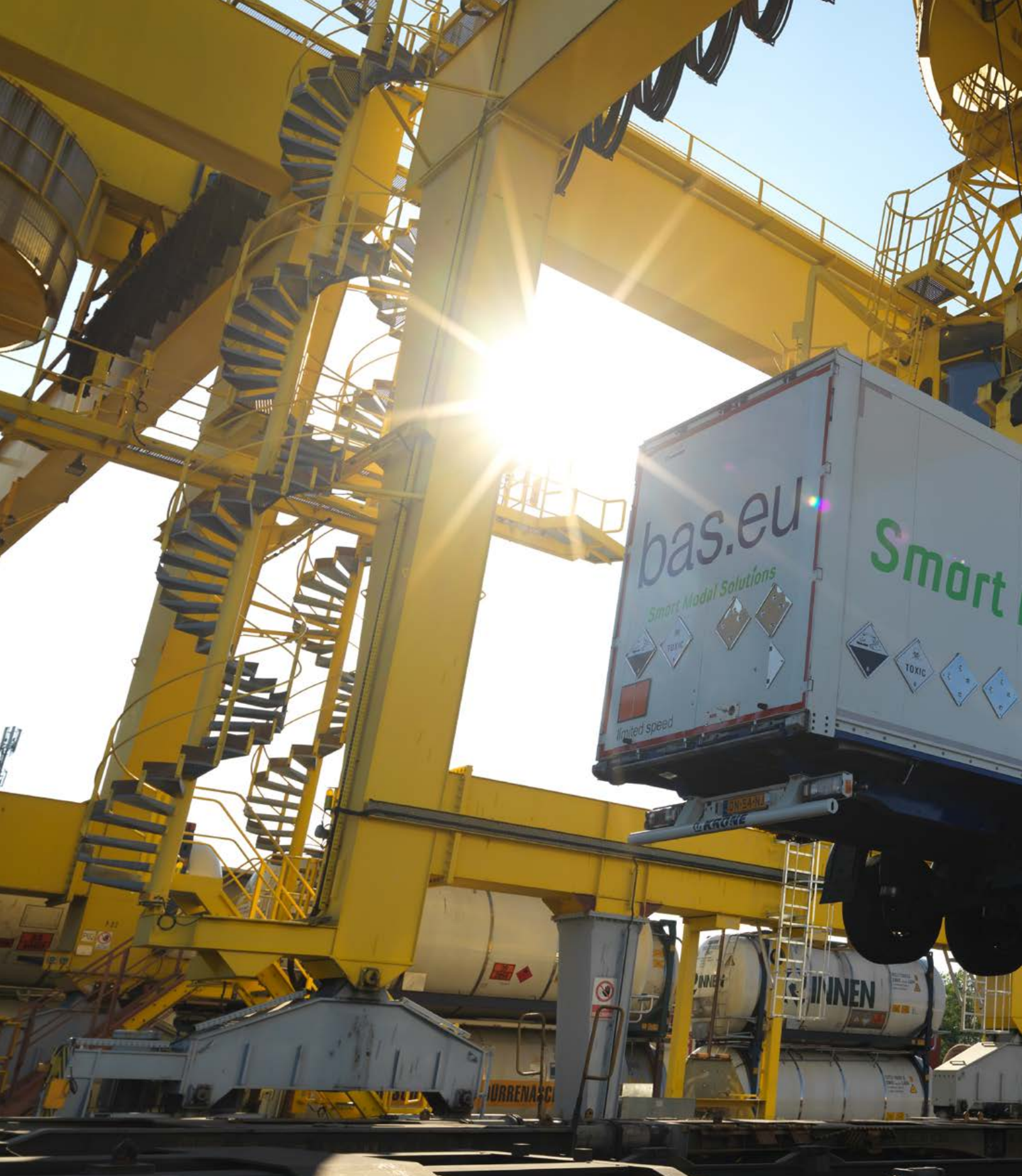
4:46 p.m.: ... the trailer hovers above the train wagon – a pocket wagon with a trestle height-adjustable to three levels.
