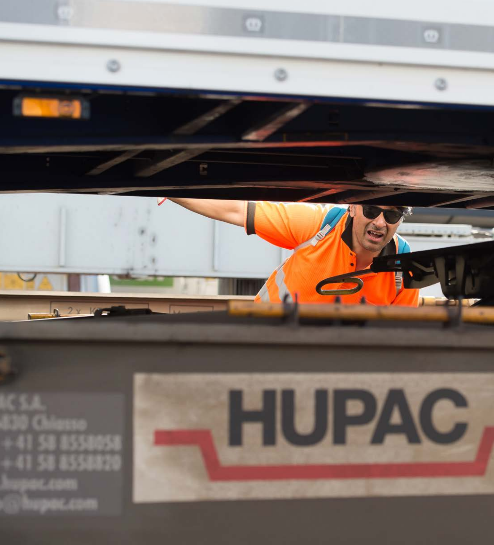
4:47 p.m.: Terminal staff member Emanuele Bazzano makes sure that the semi-trailer's centre kingpin has been latched correctly to the saddle. Using hand signals and a walkie-talkie he gives the crane operator instructions down to the last centimetre.
