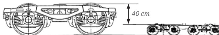
Comparison of bogie types: a 2-axle flat or pocket wagon bogie (left) and a 4-axle RoLa wagon bogie
