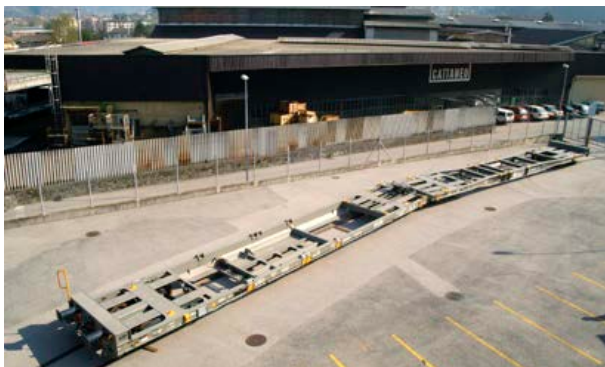
A 2 x 4 axle Mega II double-wagon unit, 2004
