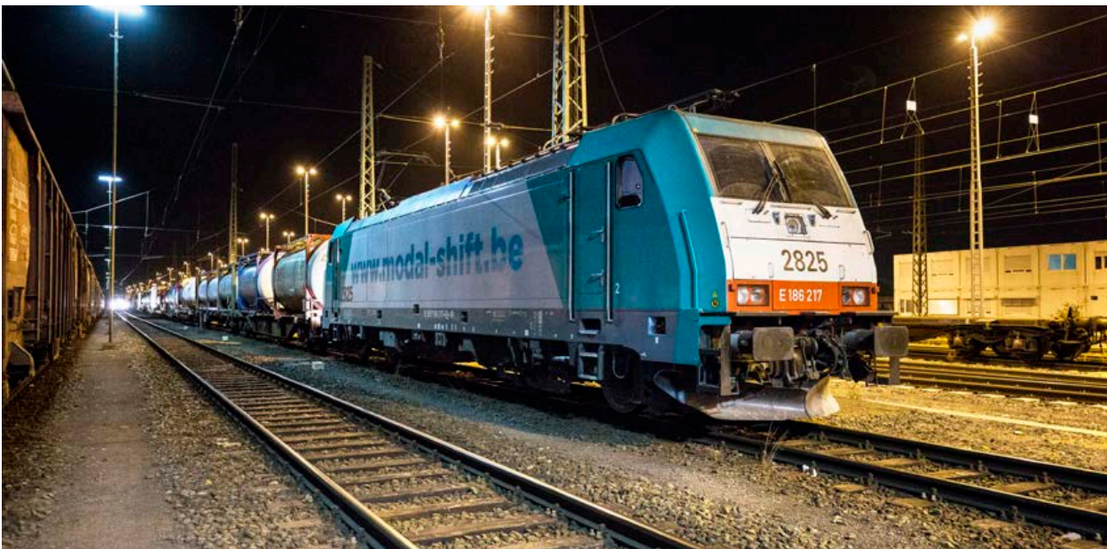
3:51 a.m.: Arrival at the goods station Aachen West. Another change of locomotive, engine driver and direction: the SBB locomotive that has hauled the train “backwards” from Cologne to here is now uncoupled. A Bombardier Traxx-series HLE28 belonging to the Belgian Hupac partner company B-Logistics couples on to the front of the train. The engine driver is likewise Belgian. At 4:48 a.m. the train continues on according to schedule ...
